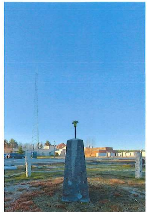
Alfred, York County - 2331N1, view looking southwesterly - Date: Nov. 9, 2021. Note that the sighting target is just the 1" diameter solid brass rod and that the green thing on top is the JAVAD Triumph-2 attached to a custom made clamping assembly.
